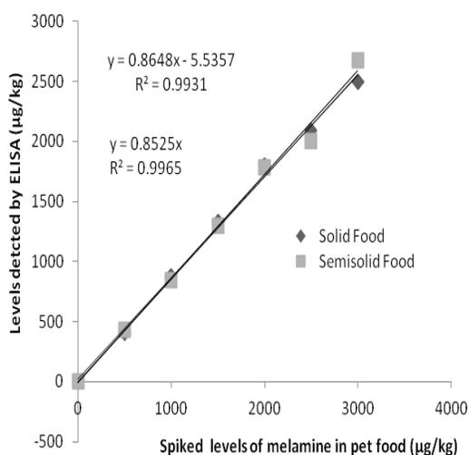
Fig. 1. Linear regression equation for melamine spiked samples solid and semi-solid pet food samples.
