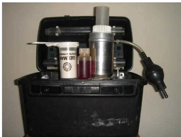
Fig. 1. Del-Agua water testing kit used for water testing.
